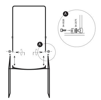
Lift each armrest a bit, then turn 90°, so the bracket aligns with the bracket on the back
